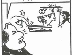
No matter how loud or soft, beautiful or ugly, all piano music is produced by pianists controlling the speed that the keys are depressed, which determines the speed that the hammers are thrown at the strings.
